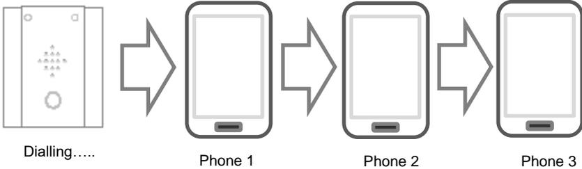
Any user receiving the call can answer, speak to the visitor, and press the following digits on their mobile or fixed line telephone to control the relays on the device...
