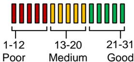
Note: Reception levels below 14 can cause problems with DTMF relay control, poor quality audio, no audio coming from the microphone on the intercom (the person on the phone cannot hear anything), or buzz on the loud speaker.
