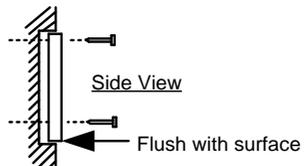
**Tip:** Use appropriate fixings to ensure the intercom cannot be removed from the wall.
