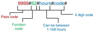
Note: This feature is only active for relay 1, and will only trigger relay 1 for the default programmed trigger time.
