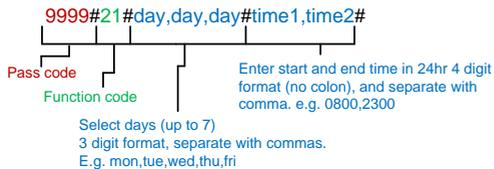
Example: to program the unit to be active between 8.00 am and 11pm, for all days send the following SMS...
