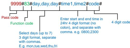
Note: This feature is only active for relay 1, and will only trigger relay 1 for the default programmed trigger time.
