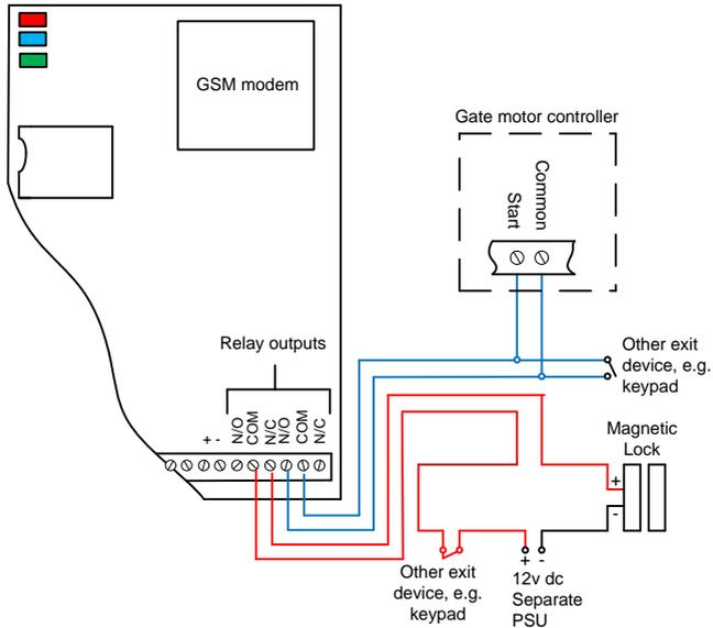
This example shows relay 1 connected to a gate motor controller for vehicle gates, and output 2 connected to a magnetic lock for a door or pedestrian gate.
