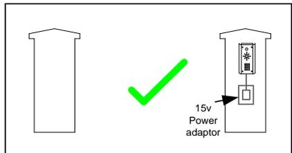
To avoid such problems, it is recommended (and is good practice) to locate the power supply as close to the transmitter as possible. This avoids power cable noise and interference and enhances the lifetime of the product.
