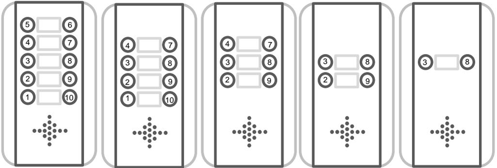
Please note the position of the buttons on the above panel options. For example, if you have a 2 button panel, you will be programming dial out numbers for buttons 3 and 8. For a 4 button panel, the corresponding button locations are 2,3,8 and 9.
